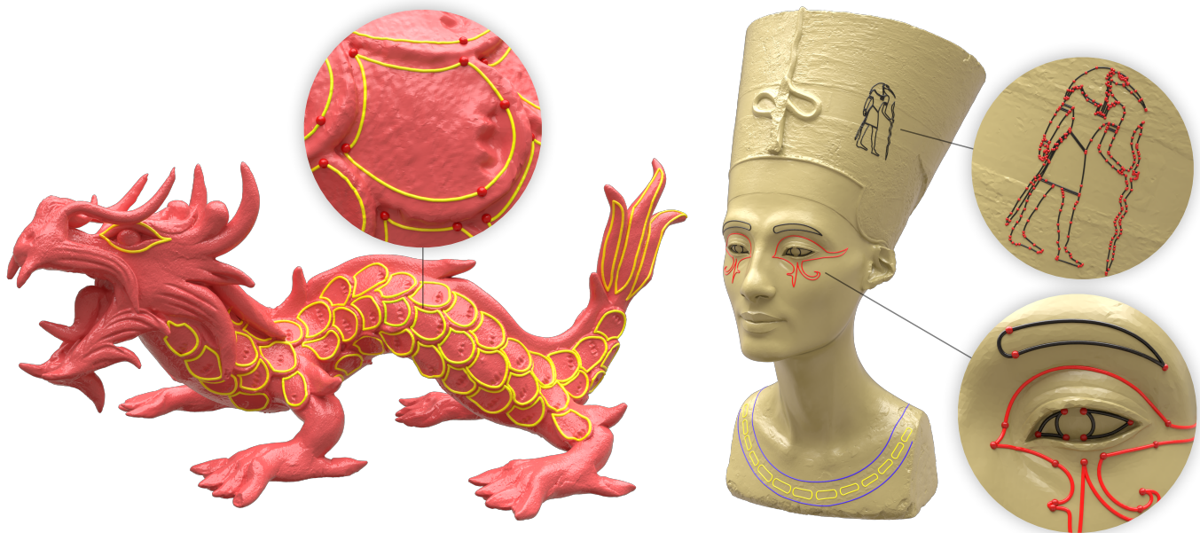
Fig. 1. We propose algorithms to interactively edit Bézier splines on large meshes, including curve editing, curve transformations and import and editing complex SVG drawings. All computations occur in the intrinsic geodesic metric of the surface. All splines in this figure have been drawn interactively. Control points and tangents of curves under editing are shown in the zoomed insets. Asian Dragon \sim 7.2 M triangles; Nefertiti \sim 500 K triangles.
